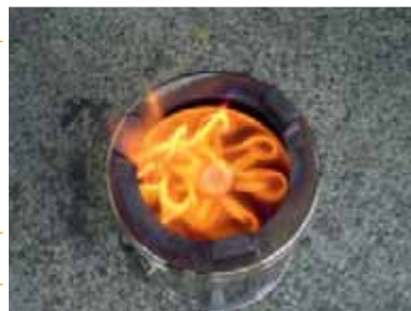
Photo 4.30 Flame pattern in the Sampada as seen from above (Samuchit)
