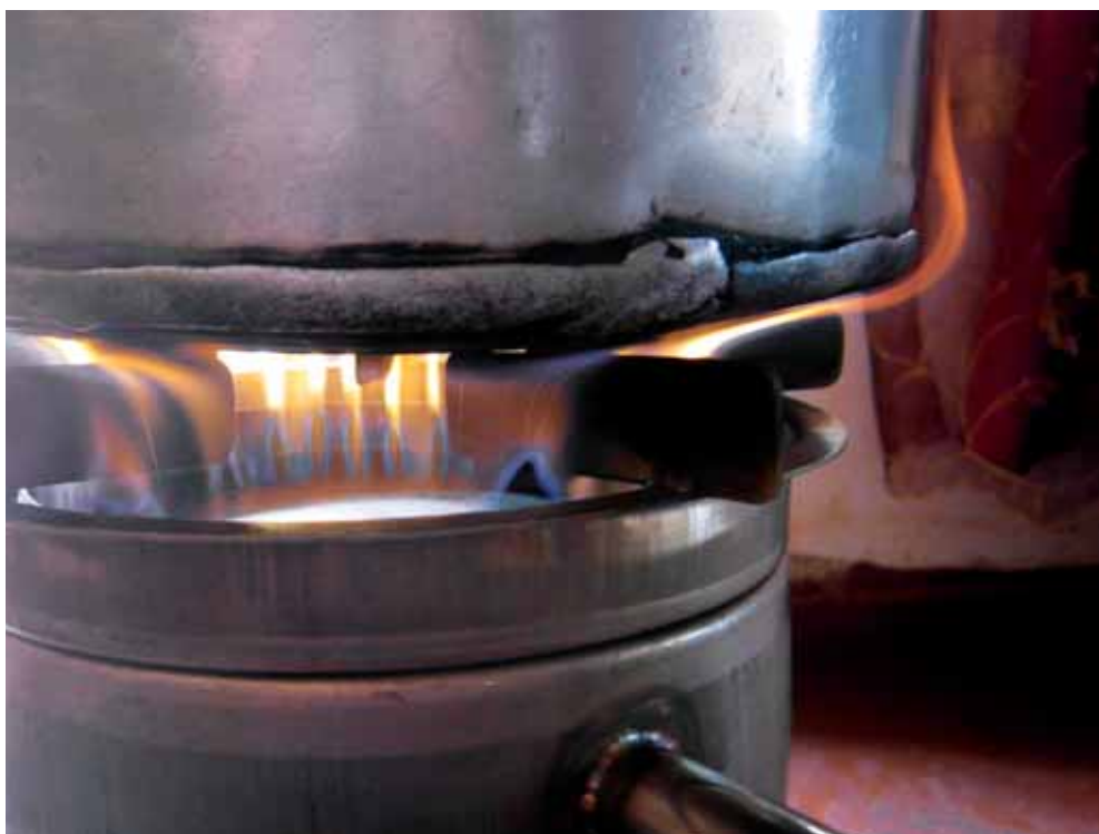
Photo 3.6 Rice husk burning with a clean flame at a residence in Malawi in a gasifier stove from Paul Olivier
