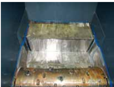
Photo 3.11 Rotating shaft with knives at the bottom of the hopper
