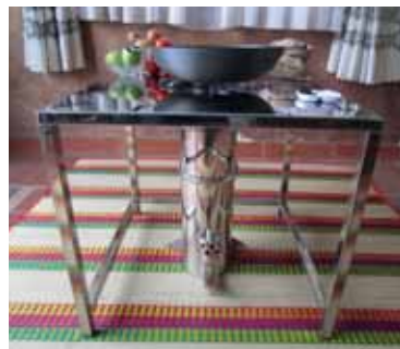
Photo 4.64 The 150 gasifier in a stainless-steel enclosure
