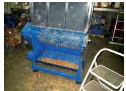
Photo 3.13 Ground material exiting through the 12 mm screen
