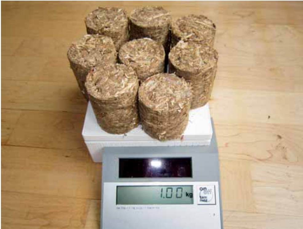
Photo 3.24 8 briquettes of 50 mm diameter from cotton stalks = 1 kg
