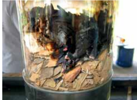
Photo 2.3 Uneven progression of an MPF due to voids in the fuel-bed increasing draft
