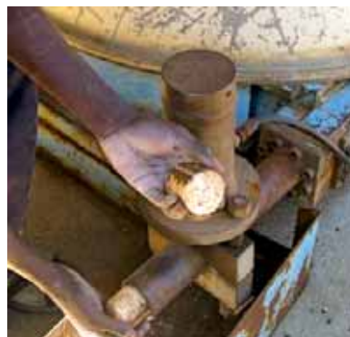
Photo 3.23 Briquette-making from saw-dust with a hydraulic press in Karamoja (Uganda) (C. Messinger)
