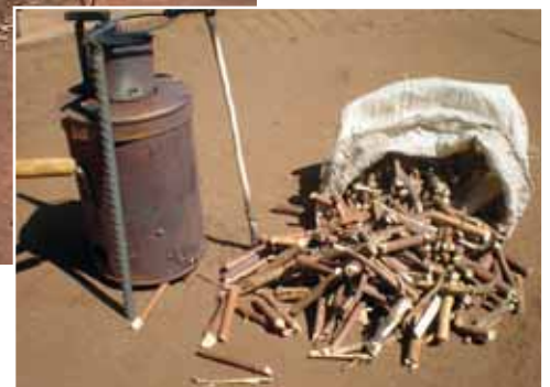
Photo 3.2 Pigeon pea stalks as a gasifier fuel for cooking: easy to break by hand or cut with a machete
